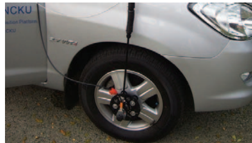
Figure 7. The distant measuring instrument was mounted on a wheel
