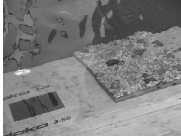
Figure 4. Different targets in water basin (assorted sizes of gravel, reflective materials), the basin offered a stepwise adaption of water depth and turbidity
