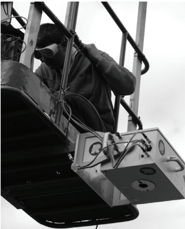
Figure 3. Lifting platform with attached breadboard system, laser and sensor orientated down to basin
