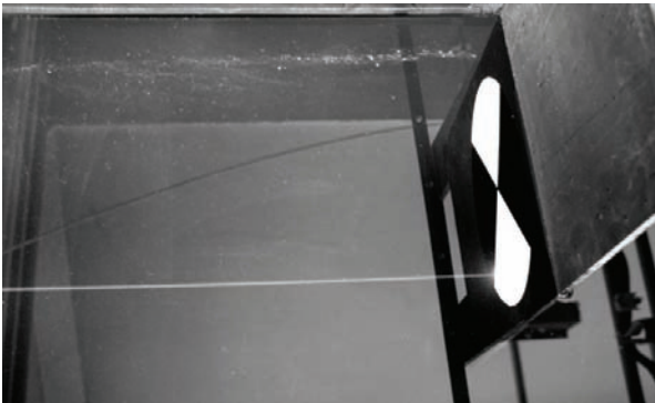
Figure 6. Hydraulic metering channel, green laser hits Secchi disk, maximum measuring depth of 16 m
