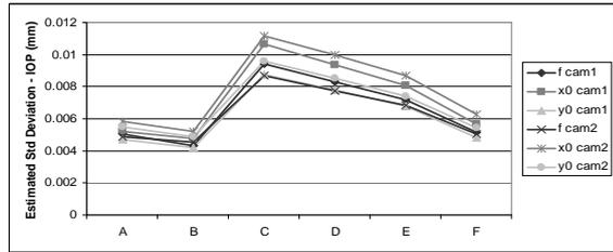
Fig. 10 Estimated standard deviations for the IOP for both cameras.
