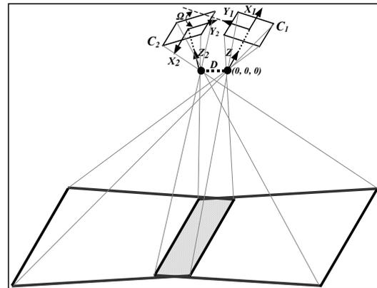
Fig 3. Geometry of a dual camera system.
