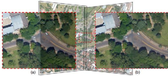
Fig. 14. Radiometric adjustment of the rectified pair: (a) before and (b) after the adjustment.
