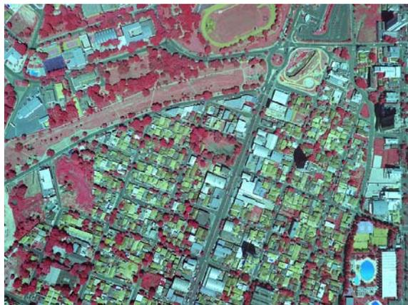
Fig. 16 Color composition generated with the two rectified oblique RGB images and one nadir IR image after rectification and fusion.
