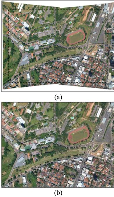
Fig. 6. Resulting fused image from two rectified images after registration (a) and, crop, eliminating the borders.
