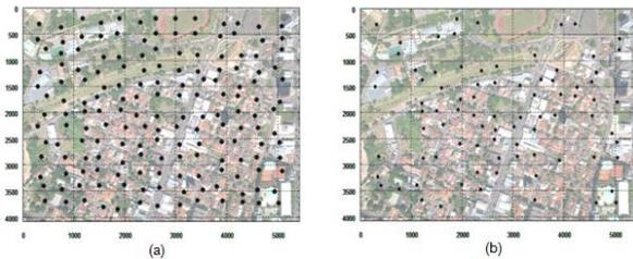
Fig. 15. (a) Interest Points automatically select by the Harris operator and (b) points used after residual analysis.
