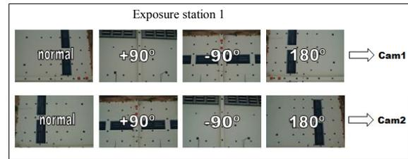
Fig. 8 Images acquired in the first exposure station.
