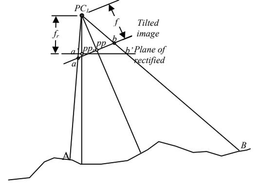
Fig. 4 Geometry of image rectification.
