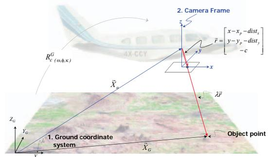
Figure 1. Coordinate systems and involved quantities in the point positioning equation based on indirect georeferencing procedure.
