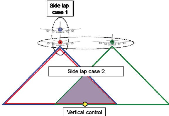
Figure 3. Optimum flight and control configuration for the estimation of the photogrammetric system mounting parameters.
