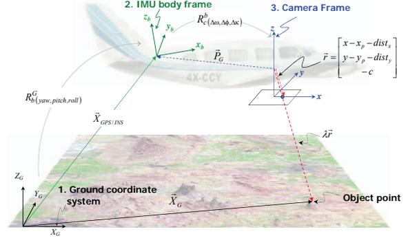
Figure 2. Coordinate systems and involved quantities in the point positioning using GPS/INS-assisted photogrammetric system.
