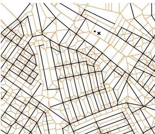
Figure 4. The LSVD of a road network.
