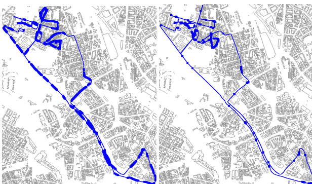
Figure 7: Results of the manual assesment for run 2 (12 km). Bold trajectory points mark erroneous positions. Left: GPS trajectory. Right: Result of matching.
