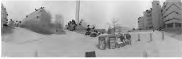
Figure 1: An image with green dots drawn on it to show the sparse 3D points found during calibration using SURF.
