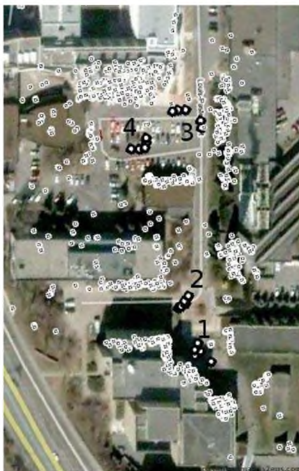
Figure 11: A mapping of the 3D points found in Sets 1 to 4. The positions of the cameras are shown as black squares with white in the middle and the 3D points are shown as white circles with black in the middle.
