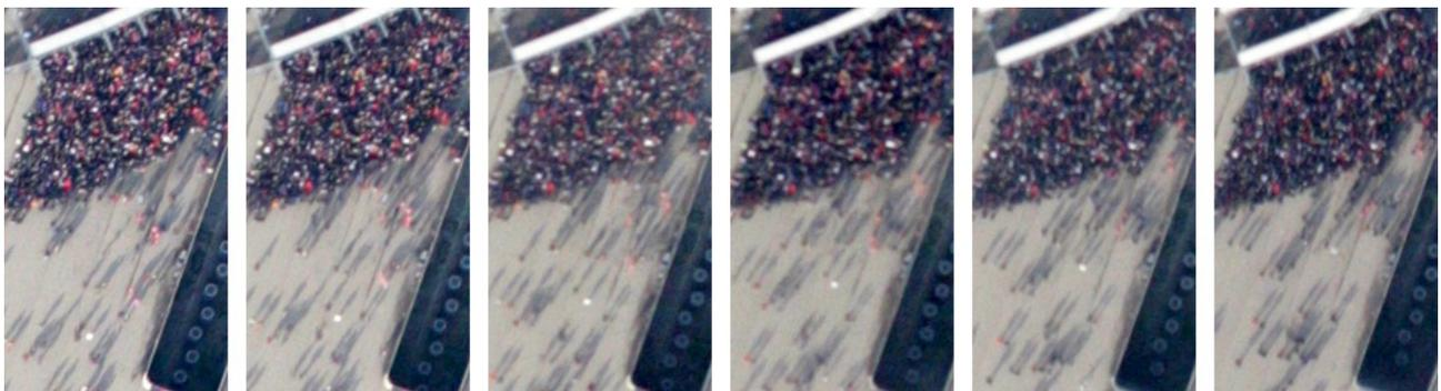
Figure 6. Test area in the aerial image sequence used for evaluation of the tracking and interpretation system; frames no. 1, 4, 7, 10, 13 and 16 out of 16 consecutive images are shown [3K-images are provided by the German Aerospace Center (DLR)].
