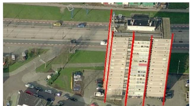
Figure 7 Lines defined by 2D corner points and approximate height projected to an image
