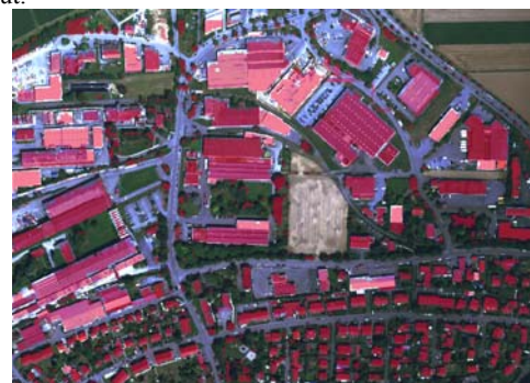
Figure 10. Building detection result (red) from method 4 (Vaihingen).
