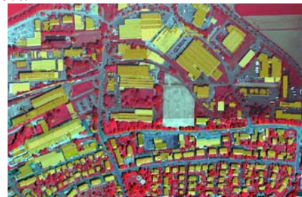
Figure 5. Building detection result (yellow) from method 2 overlaid on CIR orthophoto (Vaihingen).
