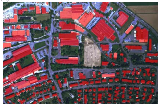
Figure 14. Final building polygons overlapped with orthophoto (Vaihingen)
