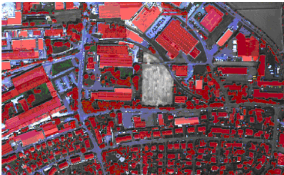
Figure 2. The detected off-terrain objects (mainly buildings and trees) after filtering
