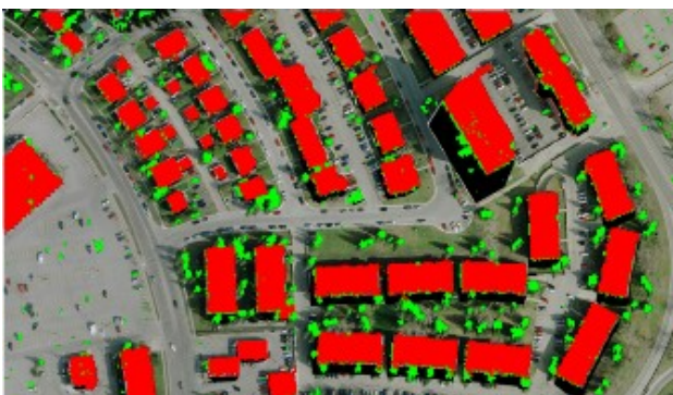
Figure 6.c. Classification results over aerial image of area (II). (red for buildings, green for vegetation, and the rest is ground)
