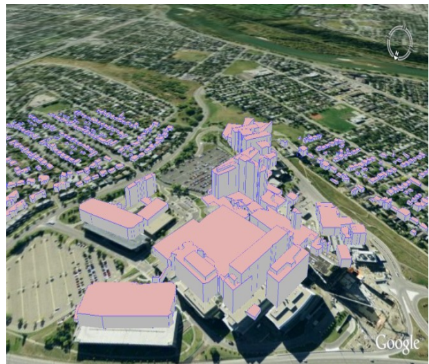
Figure 7. 3D model of the entire data set rendered over Google Earth scene of test area using COLLADA language.
