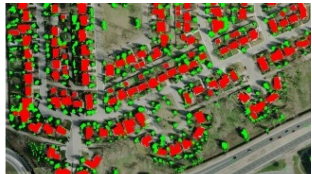
Figure 5.c. Classification results over aerial image of area (I). (red for buildings, green for vegetation, and the rest is ground)
