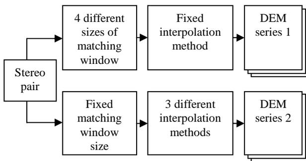
Figure 1. Method of DEM reconstruction with variable matching parameters and interpolation algorithms
