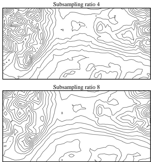
Figure 8. Contour lines generated with different mesh size DEMs
