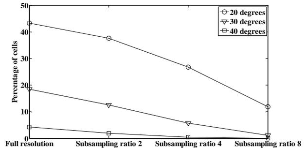
Figure 6. Percentage of cells with slope greater than 20, 30 and 40 degrees for different mesh sizes
