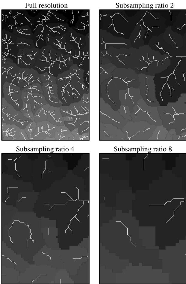
Figure 7. Stream networks and watersheds extracted from DEMs with different mesh size
