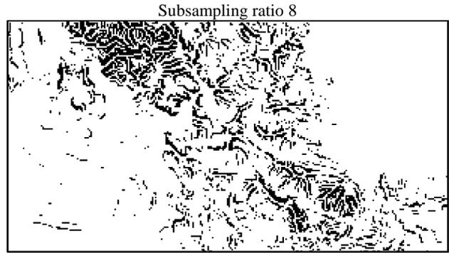
Figure 5. Slope cells with values greater than 20 degrees derived from degraded DEMs (in black colour)
