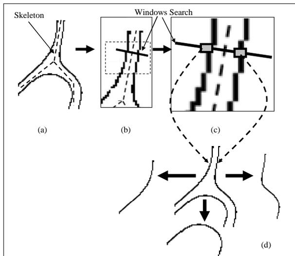
Figure 05 - a) Edges with skeleton b) Search windows unidimensional c) Seek edge pixel based on one-dimensional search window, d) Edges of the selected region of crossing.
