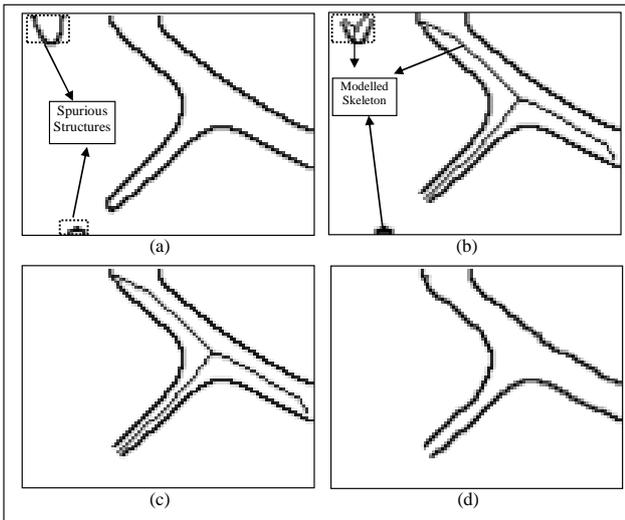
Figure 04 - (a) Edges extracted from the binary image, (b) Edges with their skeletons modelled, (c) Result of filtering the skeletons with their edges, (d) Edges selected based on the skeleton filtered.
