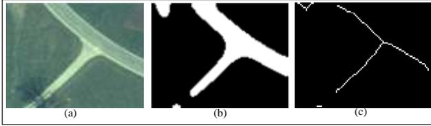
Figure 02 - (a) Original image of road crossing, (b) Segmented Crossing (binary), (c) Skeleton of the region of crossing.
