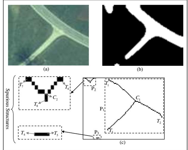
Figure 03 - (a) Original image, (b) Binary image, (c) Skeleton modelled and with their spurious structures.
