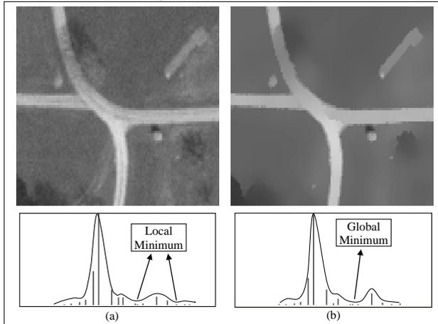
Figure 01 - (a) original image and its histogram, (b) Smoothed Image and its histogram.
