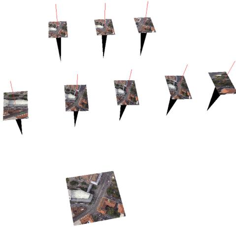
Figure 2: Overlapping camera positions mapping the same scene on ground. The derived range information and camera data are used to compute corresponding pixel locations in the perspective images.
