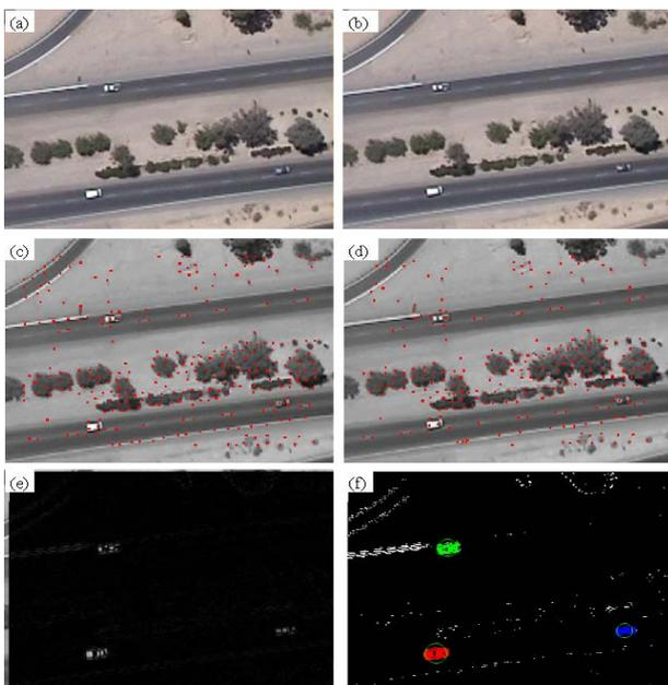
Figure 3: Moving target detection and speed measurement from two consecutive frames of an aerial video sequence with three moving car.
