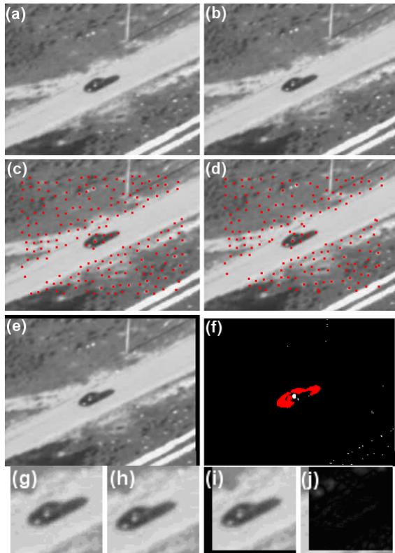
Figure 2: Moving target detection and speed measurement from two consecutive frames of an aerial video sequence with one moving car.
