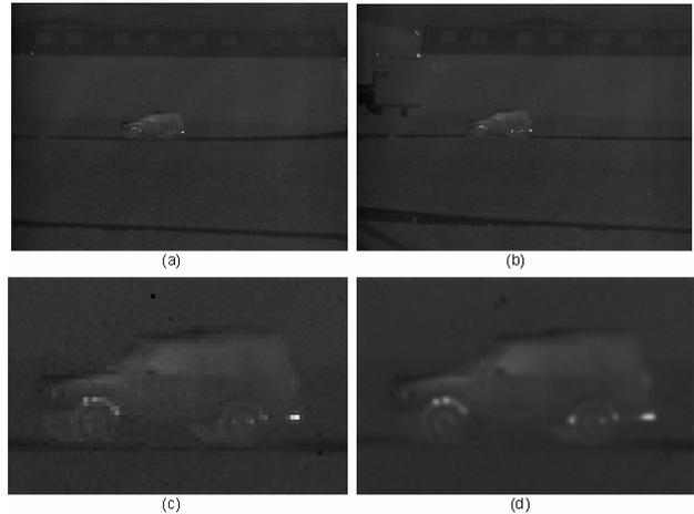
Figure 4: SRR of a thermal video image sequence of a moving vehicle. (a-b) Frame 1 and frame 30 extracted from the video with 314×233 pixels. (c) The image (76×49 pixels) of the moving vehicle extracted from frame 1. (d) The SRR result produced from 30 frames.
