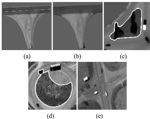
Figure 9. Failed and imprecise island extraction due to poor contrast (a, b), shadows (c) and heterogeneous road surface and islands (d, e).
