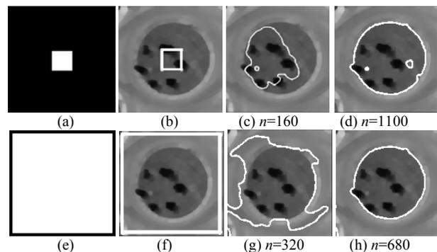
Figure 4. Initialization and curve evolution, with  $n$  denoting the number of iterations: (a) initial level set function; (b) initial curve situated inside the island; (c) intermediate result of curve evolution; (d) evolved curve; (e) initial level set function; (f) initial curve located outside the island; (g) intermediate result; (h) evolved curve.
