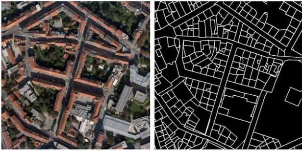
Figure 1: Test area in Graz of 400 m x 400 m, with orthophoto (left) and cadastral map (right). We find here 221 buildings on 336 properties.
