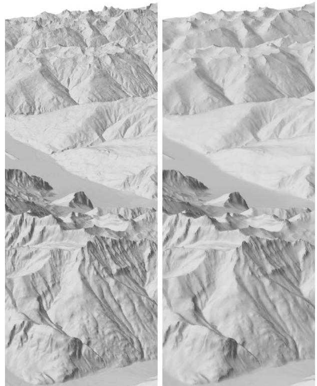
Figure 4. Increasing filtering from foreground to background. Left: original terrain; right: filtered terrain, with ridges accentuated in the background.
