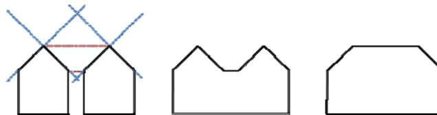
Figure 10. Front-view of two saddleback building models and their cell decomposition (dashed blue lines) and two possible aggregation results.
