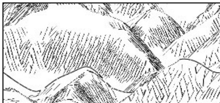
Figure 11. Maximum line width of 3 points. Line width attenuation is weighted by 90% for absolute slope, 10% for lighting. The flat hilltop at the upper left is bright.
