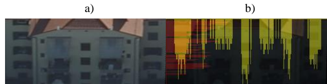
Figure 7: To the left is a rectified facade image with a depth structure, to the right a failed count of windows. The 3D structure needs to get considered.
