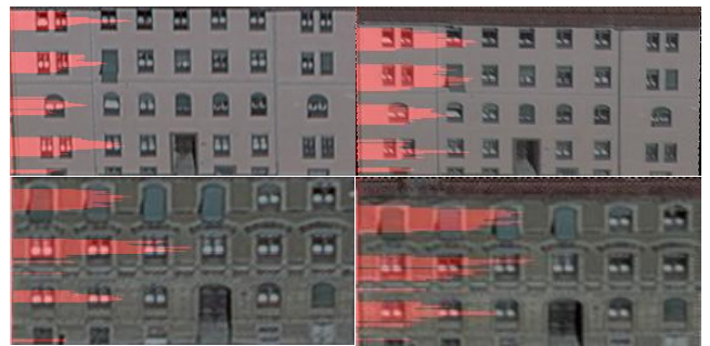
Figure 4: Two examples for floor detection using edge histograms. The oblique images are to the left.
