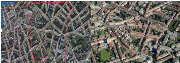
Figure 1: Detail from Microsoft Bing Maps. Left is the orthophoto and superimposed the outline of an oblique aerial image produced with the Pictometry system operated by Blom [www.blom.no]. Right is the oblique aerial image.
