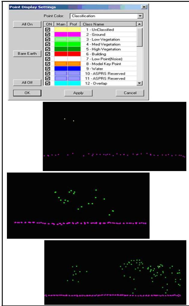
Figure 4. Profile Analysis Illustrating Ground and Vegetation Classification
