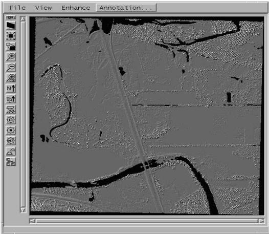
Figure 1a. DSM Created from LAS Points
