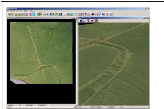
A useful viewing technique is to look at profiles to see landscape variations in the data. The profile analysis in Figure 4 shows that ground and vegetation points are reasonable. The different colors indicate the assigned classification.
