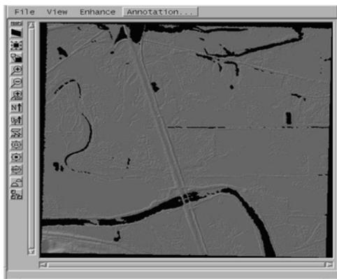
Figure 1c. DTM Voids Filled With Inpainting
