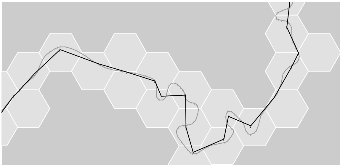
Figure 1. Generalized approximation. Input line vertices are in grey. Output vertices are located in each hexagon at the mean x-y coordinate pair calculated from the input vertices in that hexagon. These vertices, as well as the resulting line, are in black.
