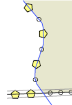
Figure 7. Alternating boundary symbology. A minor civil division is on the left, sharing a boundary with an incorporated place on the right.
