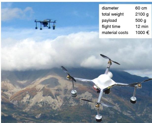
Figure 2. Modified Mikrokopter-system
