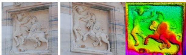
Fig. 4. Automated 3D reconstruction of a marble bass-relief (ca 1.5 m width) modelled from 5 images. The dense matching of CLORAMA produced a DSM with a 1 mm grid resolution and ca 2.3 million points.
