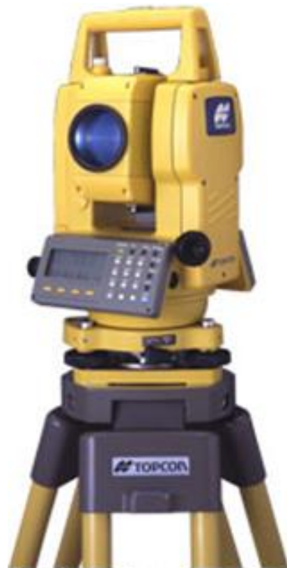
Fig 2 Topcon 3007 total station
