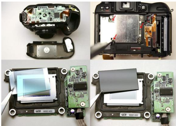
Fig. 3. Replacement operation of black filter
