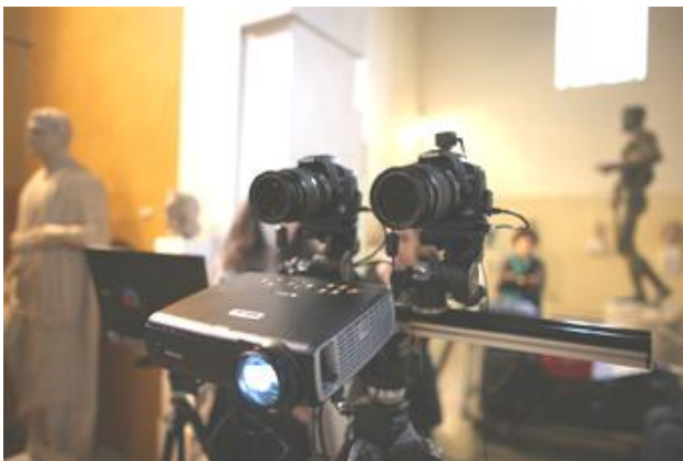
Figure 3: The main components of the SL2 scanner
