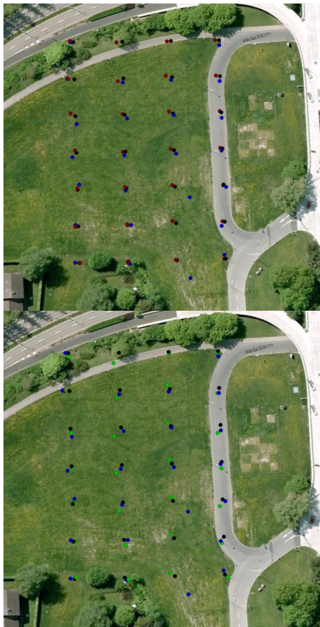
Figure 8: Flight performance during the accuracy test. Black dots are the planned image positions; Left: Red/Blue dots represent the acquired position with 1m/2.5m accuracy level respectively. Right: Blue dots illustrate stop points with 5s dwelling time and green dots represents 0s dwelling time (cruising mode).
