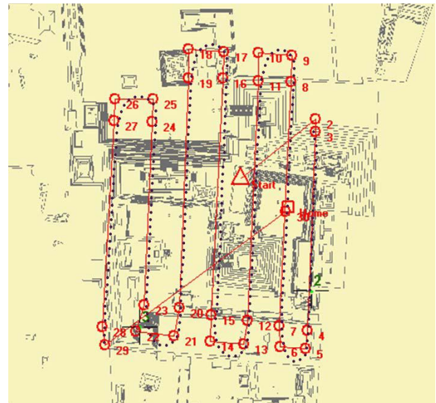
Figure 3: Comparison of the mission integrated into the flight control system (wePilot1000) and the flight trajectory. The red line shows the planned mission, including start and home point. Black dots illustrate the acquired image positions.
