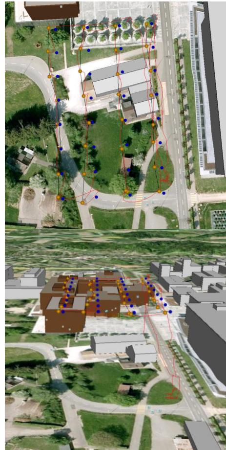
Figure 7: Flight performance of the Falcon 8 during the data acquisition at the Science City Campus Zürich visualized in Google Earth: Blue dots show the planned image acquisition points; The orange dots represent the image position obtained with the Falcon 8 system; The red line illustrates the flight trajectory. Left: Top-down view; Right: Inclined south-north view.
