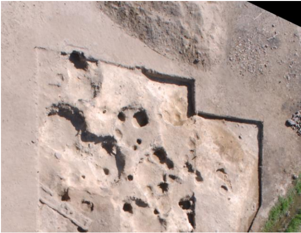
Figure 6: Orthoimage with a footprint of 0.8 cm of the excavation site. The excavation trench is clearly visible, as well as several artefacts. The visible detail allows for intra site mapping of finds down to a size in the decimetre range.
