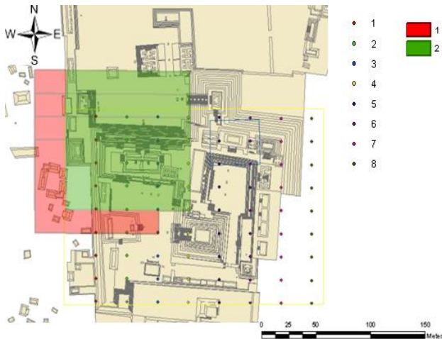
Figure 2: Visualization of the flight planning of the east and west court of Copán showing the projection centers of the individual image strips (dots) and exemplary image coverage of view images.
