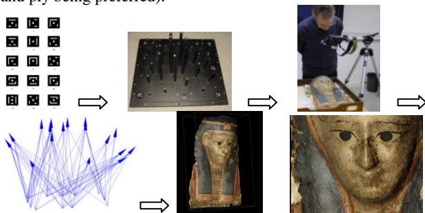
Figure 5 Image acquisition pipeline of a Petrie Museum object, a fragile cartonnage mask (UC45849). The images show: coded targets, calibration object, photogrammetry in progress, network geometry in VMS, output results as texture mapped TIN.
