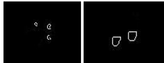
Figure 4. Left: Disconnected edges; Right: Connected edges.
