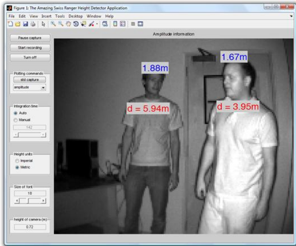
Figure 1. Screen shot from person height detection software. Average distance from the camera (labelled “d”) and object height (not labelled) is displayed on the active brightness image in real time.
