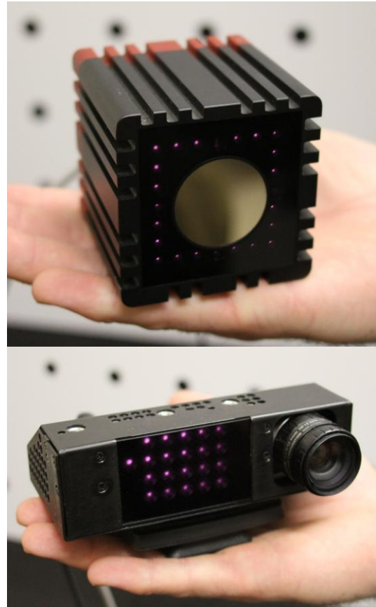
Figure 2. Range imaging cameras, SR4000 (top), and XZ422 (bottom). Note that the IR LEDs seen here as purple are not as visible to the naked eye.
