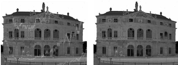
Figure 1. Imaged polar coordinates with gaps (left) and filled gaps (right)
