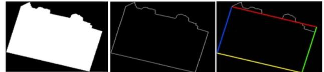
Figure 6. The classification layer “building” is based on color and texture. (a) shows the binary layer, (b) its contour in raster and finally in (c) the geometric figure of the footprint.
