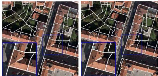
Figure 4. A cadastral vector data set is superimposed onto the true orthophoto for a segment of the Graz demo site. Note the small discrepancies between the data along property boundary lines manifesting themselves as visual feature in the imagery.
