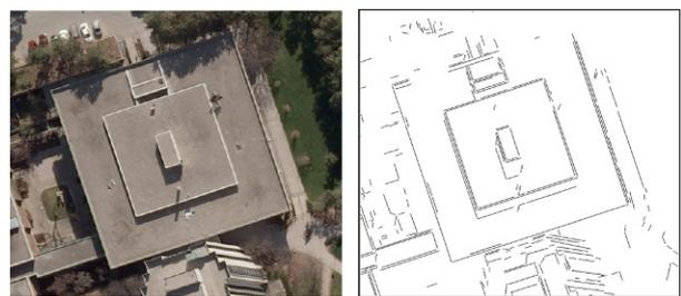
Figure 7. Extracted straight primitives (building 4)
