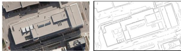
Figure 9. Extracted straight primitives (building 6)
