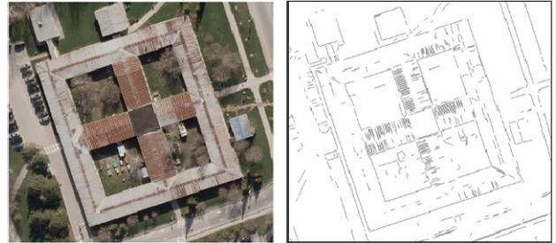
Figure 4. Extracted straight primitives (building 1)
