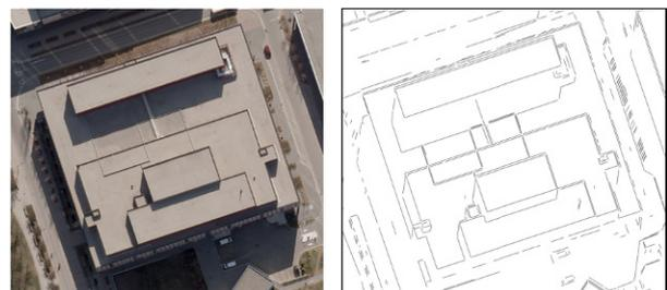
Figure 8. Extracted straight primitives (building 5)
