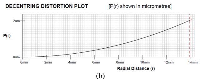
Figure 8. Decentering distortion plots showing distortion (Y-axis,  $\mu\text{m}$ ), against radial distance (X-axis, mm) for results of camera calibration obtained from (a) Cage and (b) Box. The plots are obtained from Australis software
