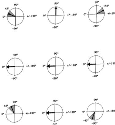
Figure 3. Camera orientations for the nine convergent image exposure stations
