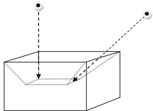
Figure 5. Camera exposure stations for box based calibration
