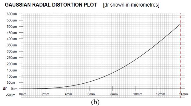
Figure 7. Radial distortion plots showing the distortion (Y-axis,  $\mu\text{m}$ ) as a function of distance (X-axis, mm) from the principal point for results of camera calibration obtained from (a) Cage and (b) Box. The plots are obtained from Australis software
