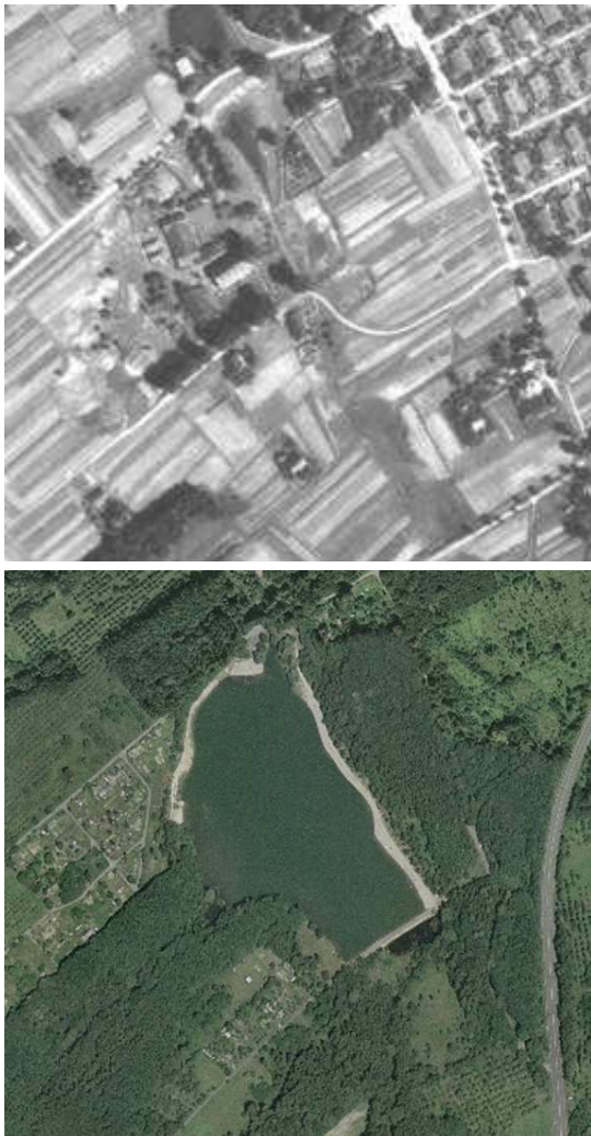
Figure 17. The area before (year 1947, © MO ČR/GeoSI AČR) and after (year 2003) the occurrence of a submerged ground subsidence
