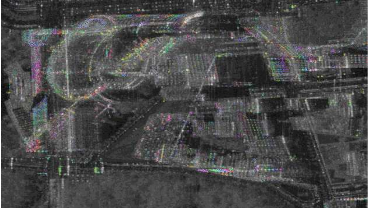
Figure 1. Phase of one interferogram of the stack overlaid on the mean amplitude image.
