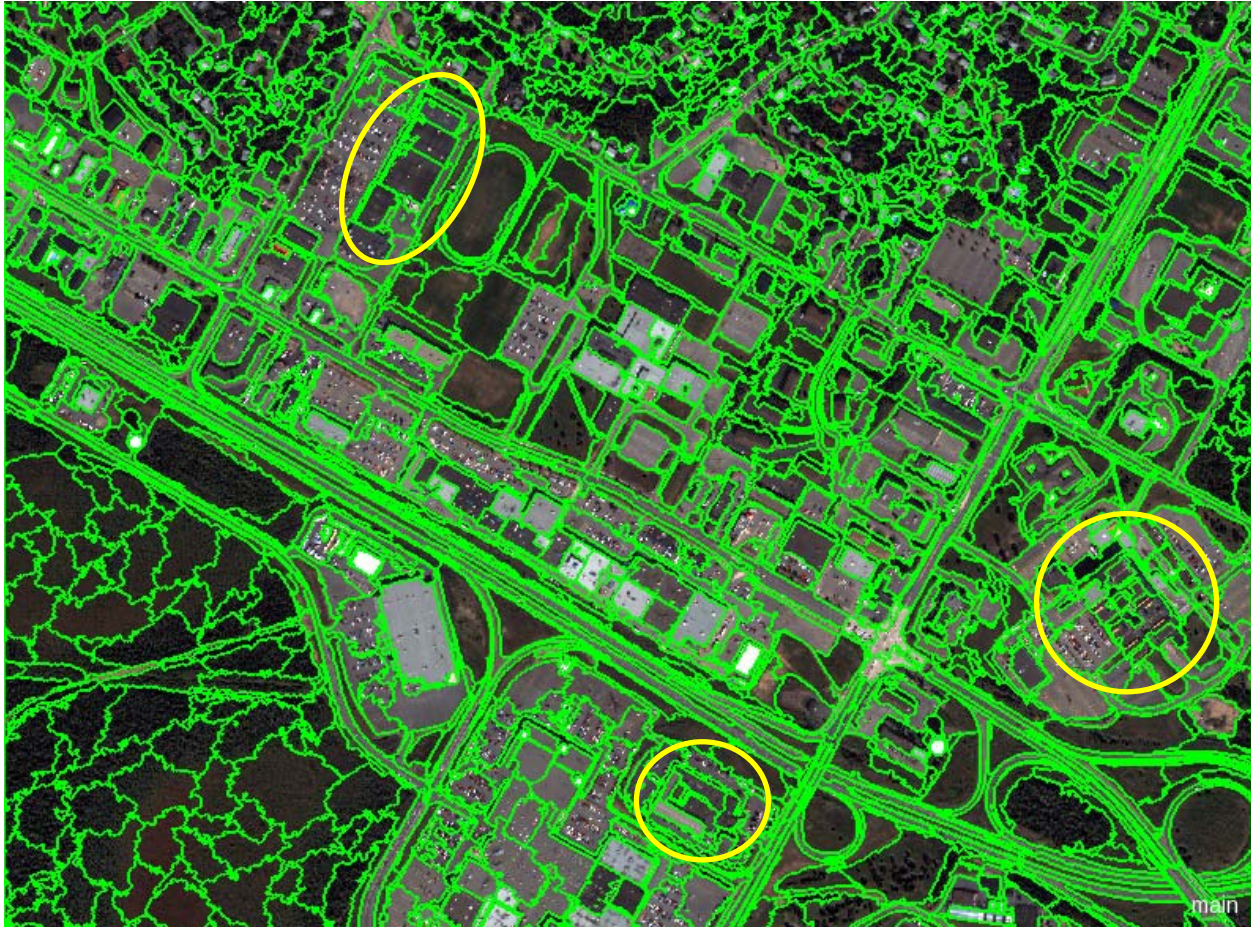
Figure 7. Segmentation result of large buildings obtained through trial-and-error parameter selection, operating time: 2 hours (pan-sharpened QuickBird MS, Fredericton)
