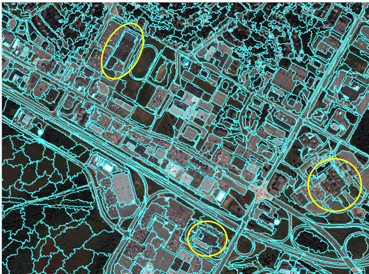
Figure 6. Segmentation result of large buildings obtained using the segmentation parameters of FbSP optimizer, operating time: 30 minutes (90% of the time was used for manual and iterative input and output of the object feature information between eCognition and FbSP optimizer, which can be reduced once the two systems are integrated) (pan-sharpened QuichBird MS, Fredericton)
