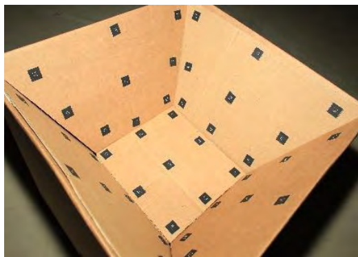
Figure 4. A rigid box design for calibration of small format cameras
