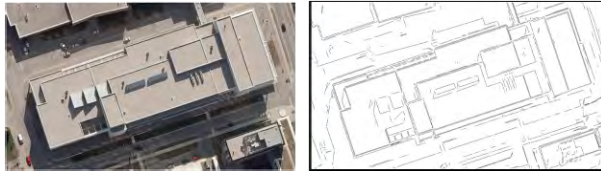
Figure 9. Extracted straight primitives (building 6)
