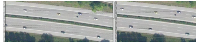
Figure 4: Tracking of a group of cars on motorway A96 near Munich. Corresponding matches are marked by dashed lines. Mind, that the motorbike was not tracked, because it was not detected (the classifier of detection was not trained to two-wheeled vehicles).
