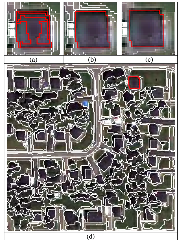
Figure 5. Segmentation process and final segmentation result using the FbSP optimizer for small buildings (pan-sharpened QuickBird MS, Oromocto). (a) Initial over segmentation using user selected initial segmentation parameters (first iteration) and the sub objects (red) selected to form a target object, (b) Target object formed by the sub objects for training the FbSP optimizer, (c) Segmentation result achieved using the parameters estimated by FbSP optimizer in the first loop (second iteration in total), (d) Final segmentation result using the parameters estimated in (c).
