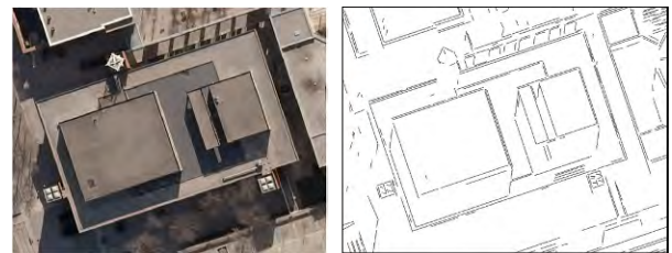
Figure 6. Extracted straight primitives (building 3)
