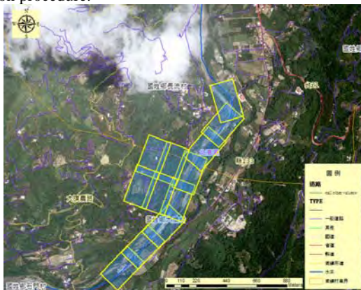
Figure1 The example of flying planning (pre-operation)
