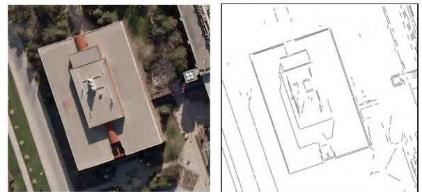
Figure 5. Extracted straight primitives (building 2)
