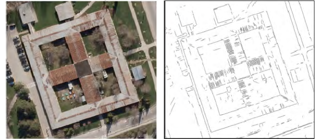
Figure 4. Extracted straight primitives (building 1)
