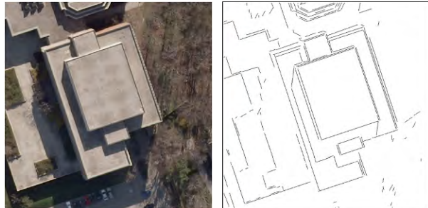
Figure 10. Extracted straight primitives (building 7)
