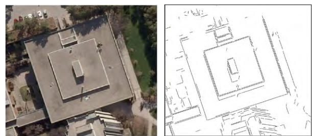
Figure 7. Extracted straight primitives (building 4)
