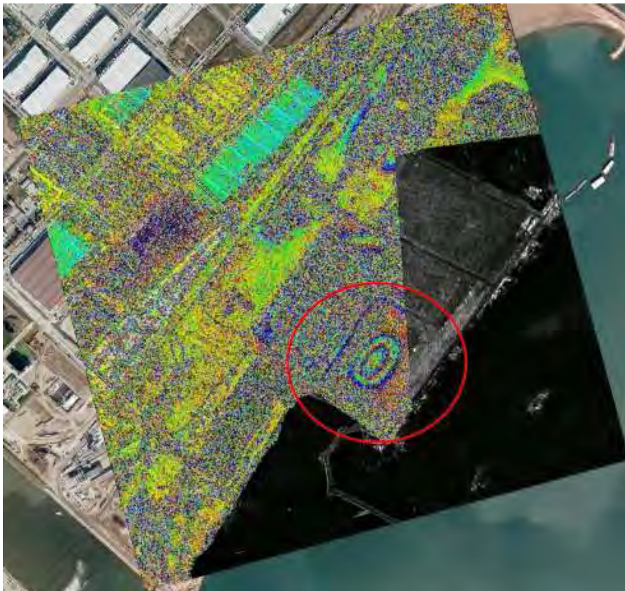
Figure 6. Example of deformation measurement based on a single interferogram. The image is a wrapped interferogram with a temporal baseline of 11 days, which is superimposed over a SAR amplitude image. Google Earth images are used as background. The red circle shows an ellipse that includes two phase fringes. The maximum deformation is approximately 3 cm. It is therefore a relatively fast deformation of 3 cm in 11 days. This result, achieved with just two images, is important especially if the high commercial price of the TerraSAR-X images is considered.
