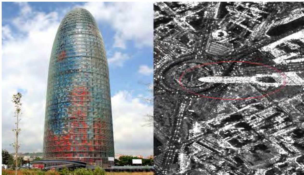
Figure 2. Example of the sampling capability of TerraSAR-X StripMap imagery. A photo of the Agbar tower, an emblematic 144 m height skyscraper of Barcelona, is shown in the left image. The mean SAR amplitude image over the same tower is shown in the right image. In this case, the mean amplitude image was obtained using 20 co-registered images. One sample every 0.75 m along the vertical direction can be obtained thanks to the resolution in range of these images (0.9094 m).
