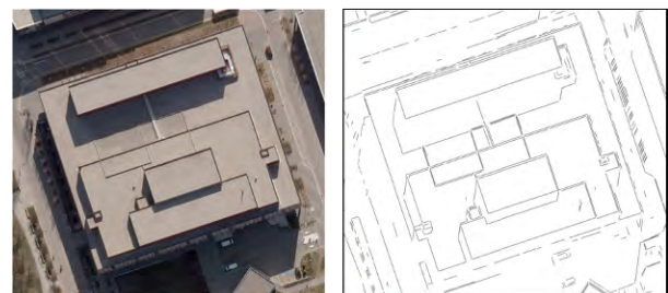
Figure 8. Extracted straight primitives (building 5)
