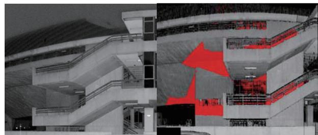
(a) The occluding scan (b) The occluded parts highlighted in red
