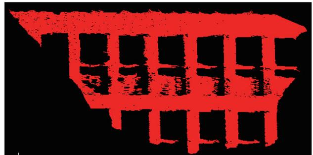
(c) The remained TIN mesh after excluding the holes and pointless triangles
