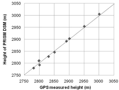
Figure 8. Validation of PRISM DSM compared with ground-based GPS height measurements
