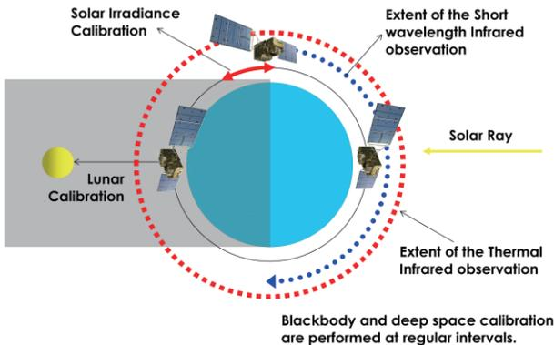
Fig. 5 On orbit operation
