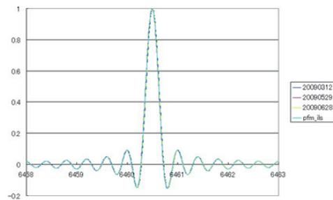
Fig. 10 Instrument function of band 2P
