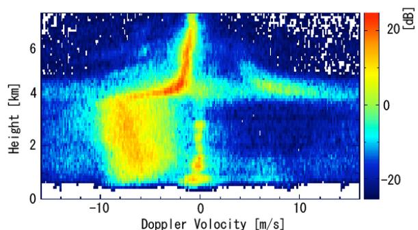
Figure 2. Doppler spectrum observed by the 400-MHz WPR
