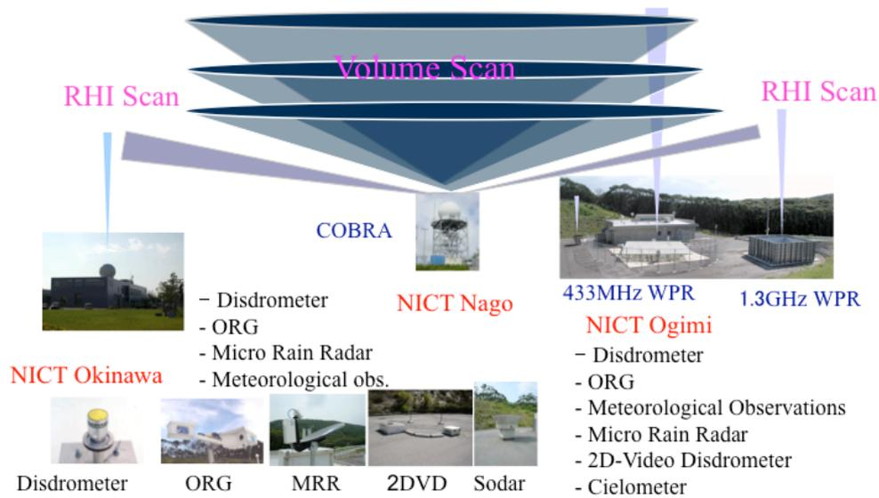
Figure 3. Outline of the intensive field observation network in Okinawa, Japan
