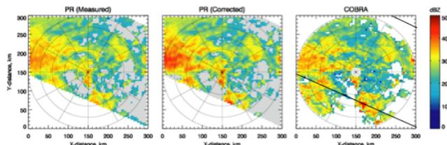
Figure 4. Comparison of horizontal radar reflectivity distribution for the PR and COBRA at a height of 2km (2004/06/09)
