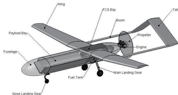
Figure 1. Josaphat Laboratory Experimental UAV (JX-1)
