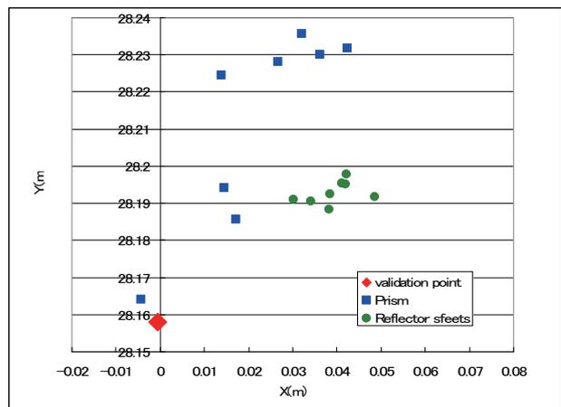
Figure 3.3. Validation point coordinates by each control point
