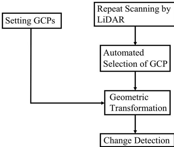
Figur1.2. Flow of LiDAR measurement for landslide monitoring
