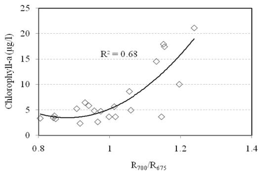
Figure 5. Relationship b/w chl-a and reflectance ratio
