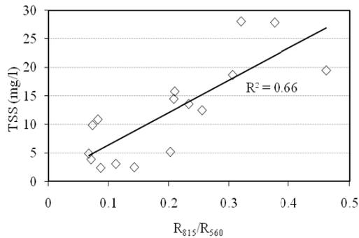
Figure 8. Relationship between TSS and reflectance ratio
