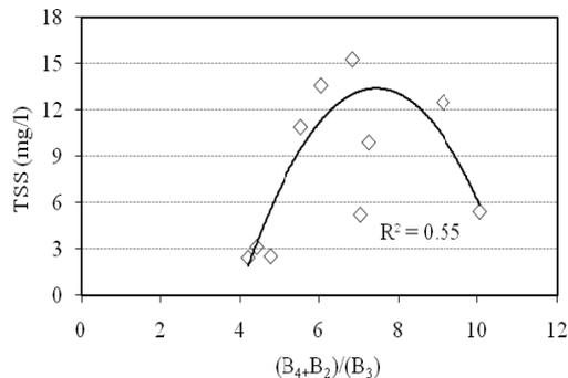
Figure 9. Relationship b/w TSS and ALOS/AVNIR-2 (3 band) reflectance ratio
