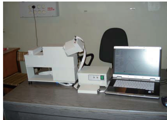
Figure 1. High precision real-time Multi-channel spectropolarimeter.
