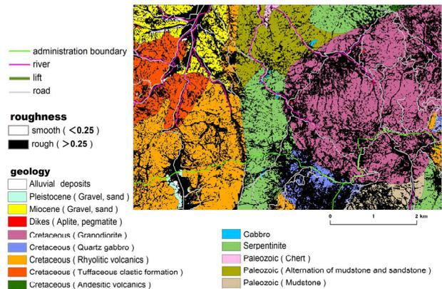
Figure 14. Overlay between geology and roughness using 1m DEM
